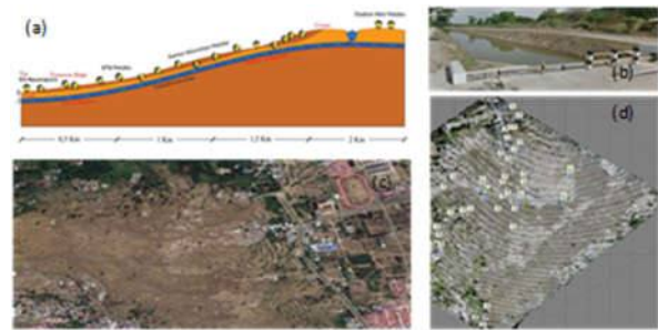
Fig. 11. (a) Model of The Collapse Mechanism of the Petobo Liquefaction Collapse, (b) Gumbasa Irrigation Canal Before The Earthquake, (c) Image of Liquefaction Aerial Flow 16 Days After The Earthquake, (d) Aerial Contour Image
